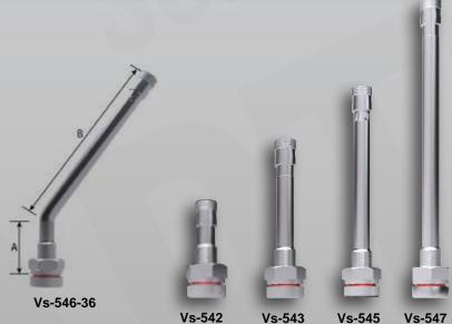
Install the valve with care and do not overtorque: the recommended torque is 7 to 10 Ft-Lb (9 to 16 Nm.)
